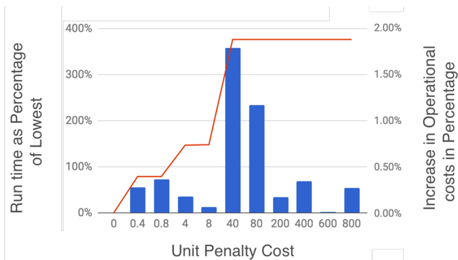
Figure 6.1: Instance AsE_10_100_4_4_95_3, run with different levels of unit penalty cost. The horizontal axis shows unit penalty cost values. The left vertical axis shows run time in percentage increase from the lowest run time, while right axis and the red graph line shows increases in operational costs as a function of unit penalty costs.
