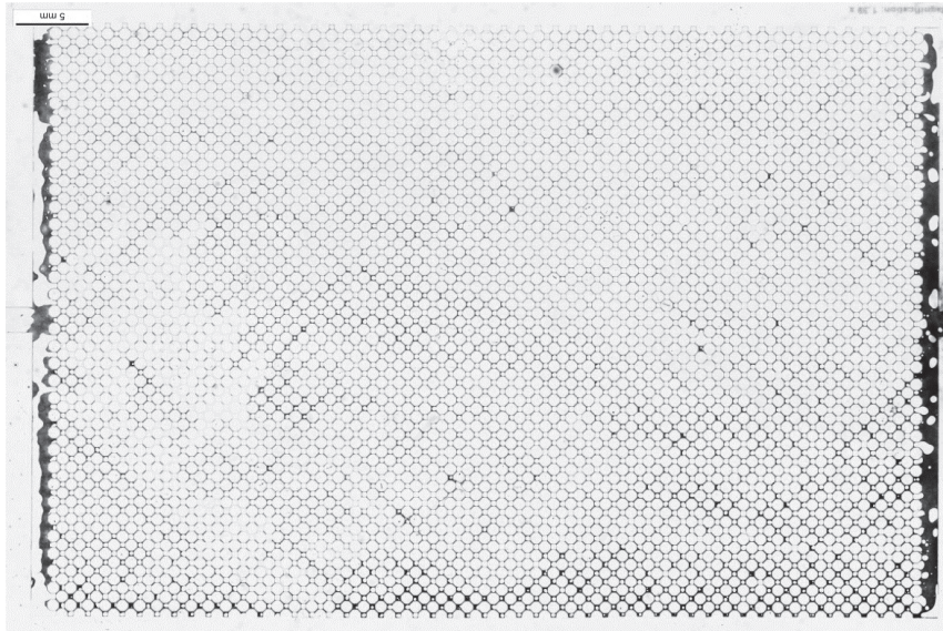
Figure H.11. Swi established after 3 PV of oil flooding. Swi is 38.7%. Flow is from left to right.
