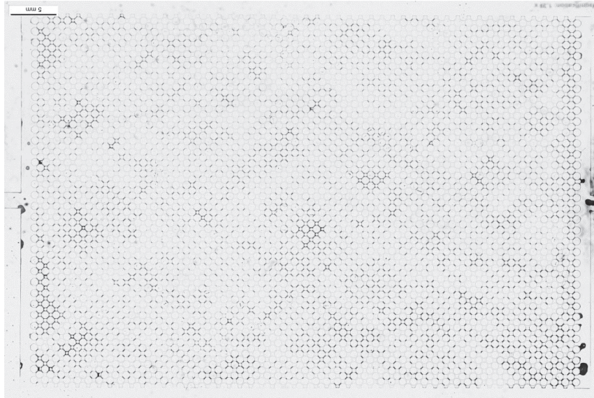
Figure H.13. S_{or_1} after 7.5 PV of water flooding at various flow rates. S_{or_1} is 28.3%.
