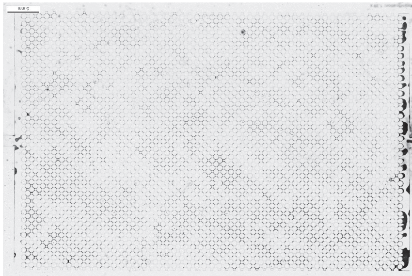
Figure H.12. After 1 PV of water flooding at 0.0025 ml/min. Oil saturation is 34.1%.
