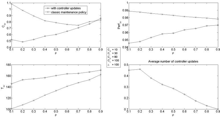
**Figure 10.**  $C_{av}$ ,  $Perf_{av}$ ,  $T_{av}$  and average number of updates vs threshold  $\rho$  for an inspection step  $\Delta = 100$
