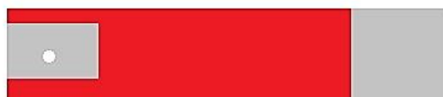
Figure 24: The geometry of test samples. The area without paint insured electrical conduction between sample and electrolyte, at the bottom, and between sample and the clamp, at the top.
