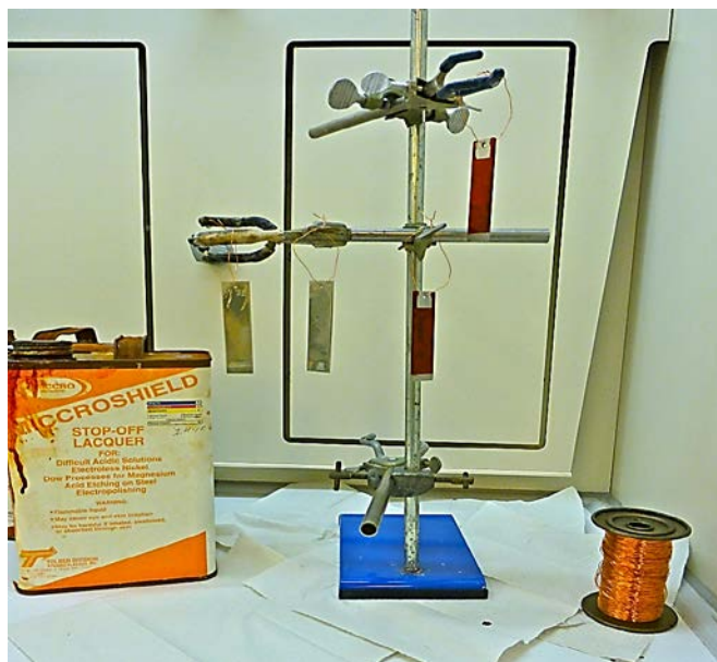
Figure 25: The coating and drying of samples took place in vented hood due to highly volatile lacquer.
