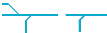
Figure 2.13: Branched and double-branched microchannel designs used in this thesis.
