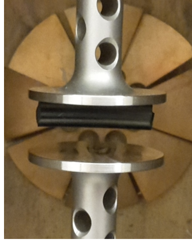
Figure 3.9: HNBR ring section adhering to one of the holders after the pull-off test.
