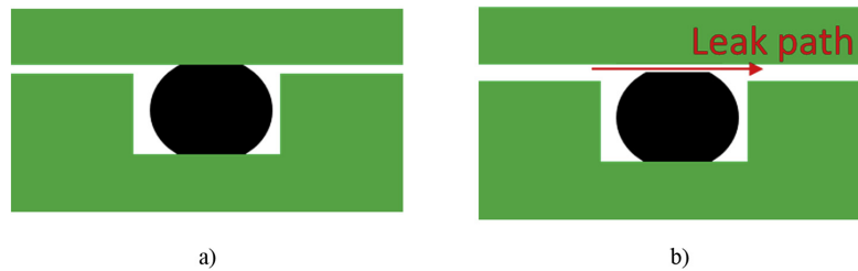
Fig. 1. Schematic of compressed O-ring seal (black) in a flange: a) at ambient temperature; b) upper part lift-off at low temperature and leakage due to “frozen” seal.
