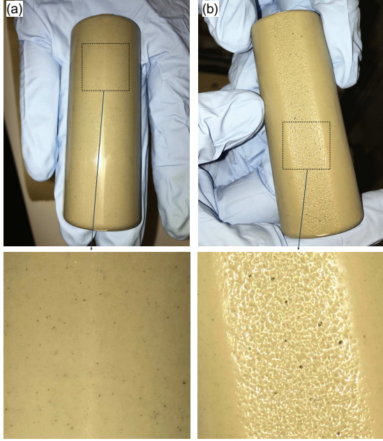
FIG. 1: Demonstration of frozen-in elastic deformation. Picture of a rubber half-cylinder at (a) room temperature and (b) at T = -40^\circ\text{C} , after the cylinder was squeezed at room temperature against a sandpaper surface, and then cooled down. Note in (b) the rectangular (nominal flat) strip of frozen-in rubber deformation (Hertz-like contact). The magnification picture (right) shows that the (nominal flat) contact area has frozen-in surface roughness inherited from the surface roughness of the sandpaper. The frozen-in deformation of the rubber cylinder stays unchanged as long as the rubber is kept at T = -40^\circ\text{C} , but disappears when the rubber sample is kept for some time at a temperature above the rubber glass transition temperature, e.g., at room temperature.
