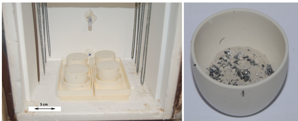
Fig. 13 Furnace with the alumina crucibles used for the phosphorus extraction using silicon metal, as well as a closeup (Color figure online)
