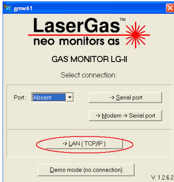
Figure A.5: The box that appears when opening the gmw61.exe program. To move on, press the LAN(TCP/IP) button.
