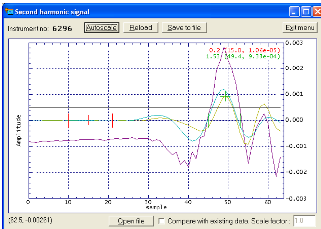
Figure A.11: The second harmonics signal of H 2 O, showing a peak at 49 on the x-axis.
