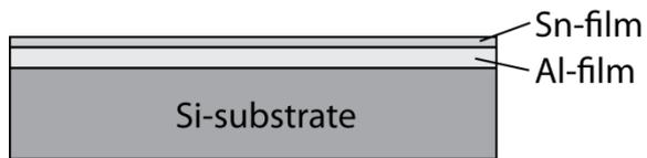
**Figure 4.6:** An illustration of the proposed protective Sn-coating for the Al-film.
