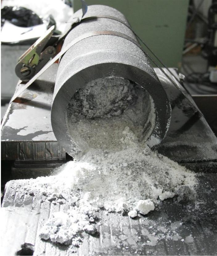
Figure 52: Failed experiment where the flux did not mix properly with the slag.
