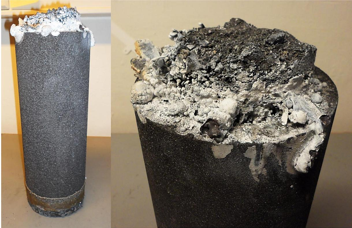
**Figure 51: Failed experiment where the top of the charge sintered into an air-tight bridge which the building CO<sub>2</sub> pressure ejected from the crucible.**
