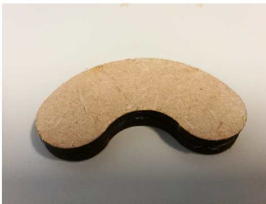
FIGURE 6 LOW RESOLUTION TOP - LASER CUT MDF
