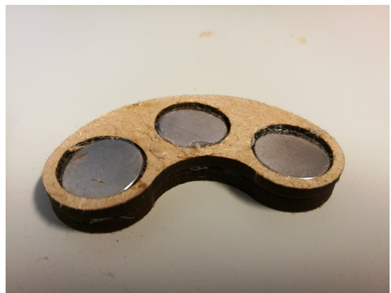
FIGURE 7 LOW RESOLUTION BOTTOM - LASER CUT MDF
