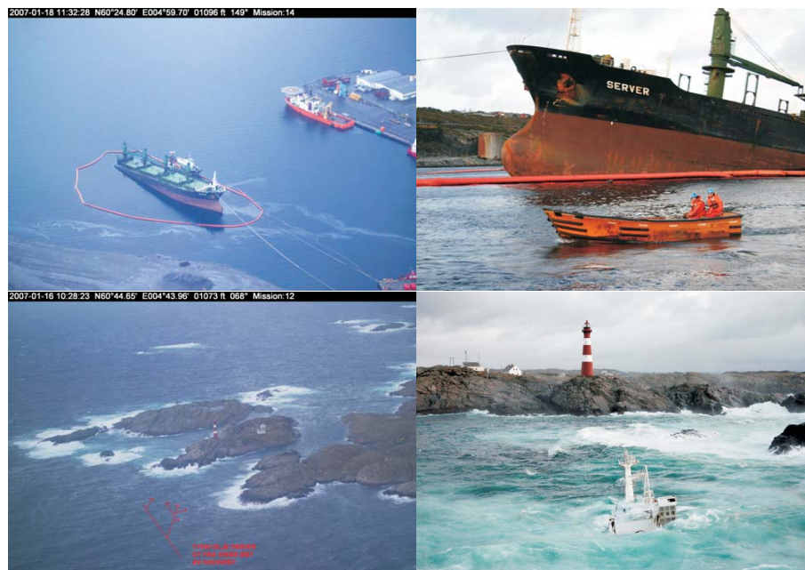
Figure 3.4: MS Server oil spill accident [ Kystverket, 2007a,b,c,d ]. She broke into two. The upper figures show the forepart of the ship, while the lower figures show the afterpart which sunk completely near Hellesøy lighthouse.
