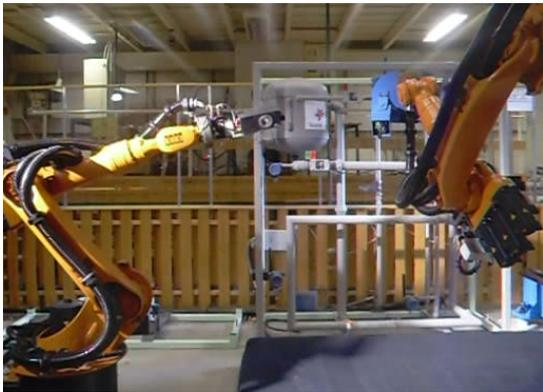
Fig. 3: The lab setup where the floor mounter robot is equipped with a stereoscopic camera.
