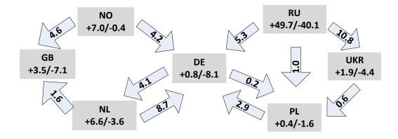
Figure 3: Natural gas network with base year data (bcf/d) for production (positive values in rectangles), consumption (negative values), and pipeline capacity.
