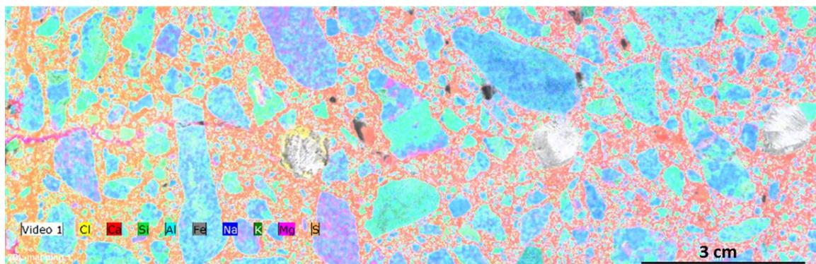
Figure 1: Elemental mapping of cracked concrete core (CC)
