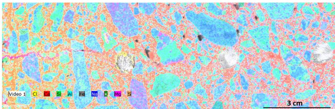
Figure 1: Elemental mapping of cracked concrete core (CC)
