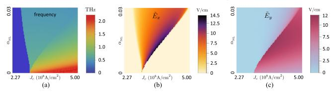
FIG. 4. Numerical results of multiple ac outputs associated with steady-state oscillations (at  $t \to \infty$ ) in the range  $J_c(10^8 \text{ A/cm}^2) \in [2.27, 5.00]$  and  $\alpha_{\text{NL}} \in [0, 0.03]$  for a NiO(1)/Pt(25) heterostructure. (a) Frequency output. (b) and (c): two perpendicular ac components (in effective values) of the electric field generated by the SHE and the spin pumping.
