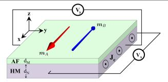
FIG. 2. An insulating AF/HM heterostructure. The applied dc current density  $J_c$  drives the AF via the SHE. The dynamics of the AF pumps spin current back into N, and converts into electric field via the inverse SHE, which is monitored by two voltmeters.
