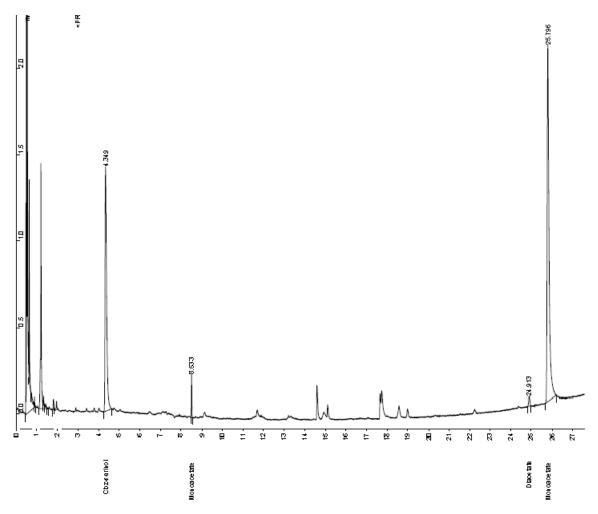
Figure 2-5: GC chromatogram of a sample from the enzymatic acetylation of 1. Temperature program: 80 - 92 °C, 30 °min<sup>-1</sup>; 92 - 98 °C, 3 °min<sup>-1</sup> (2 min); 98 - 104 °C, 3 °min<sup>-1</sup>; 104 - 140 °C, 30 °min<sup>-1</sup>; 140 - 200 °C, 3 °min<sup>-1</sup>; total time 28 min.
