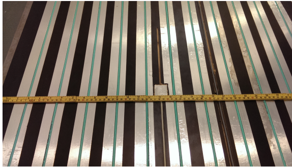
Figure 2.16: Sensor integrated into the bottom plate of the tank
