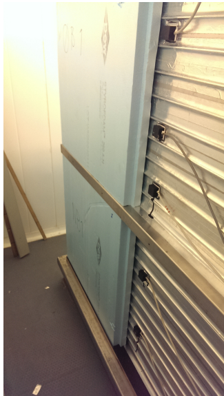
Figure 2.17: Five sensors in vertical line measuring vertical temperature profile in the tank.
