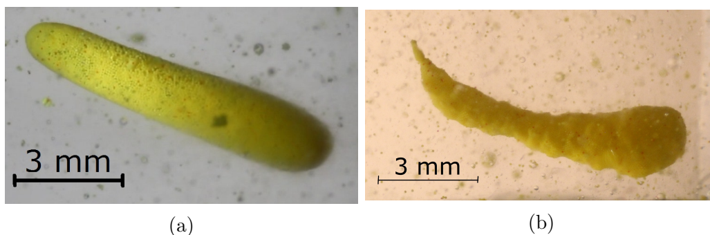
Figure 4.1: Tubes produced by applying an external electric field on droplets of volumes 30 and 50\mu\text{l} in Figures (a) and (b), respectively. The electric field operates horizontally normal to the line of sight from the microscope.
