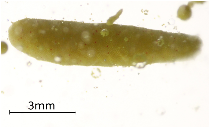
Figure 4.2: The use of pipette tips to obtain tubes of silicone oil suspended in castor oil. The particles used were PE63-75.
