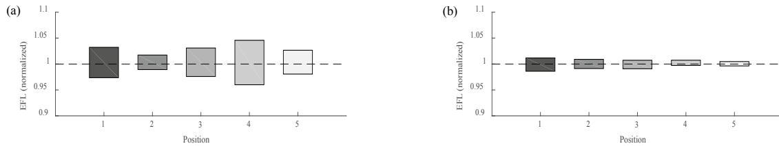
Fig. 4. Total EFL at each position for (a) v_w +/-4% and (b) TI +/-5%. The results are normalized to the design case. An increase in mean wind speed as well as turbulence intensity results in an increase of the total EFL
