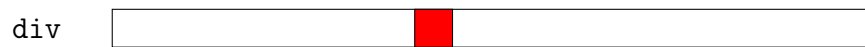
Figure 6.5: The data elements each thread is required to access in global memory in order to compute the Divergence on an unstructured grid. This is the model used in the CUDA back-end.
