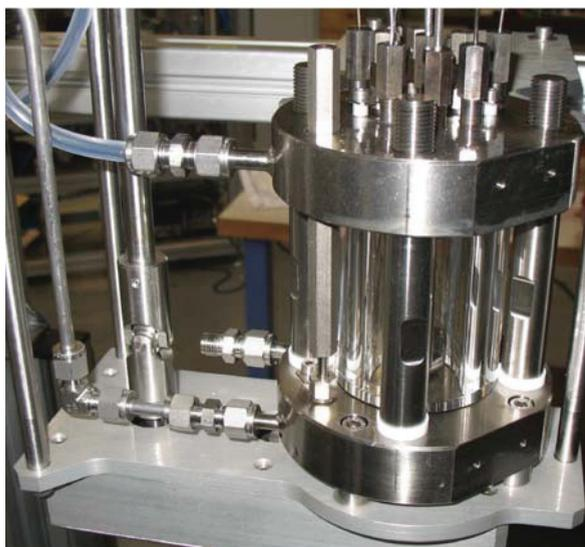
Fig. 1: The  $CO_2$ Mix VLE cell.
