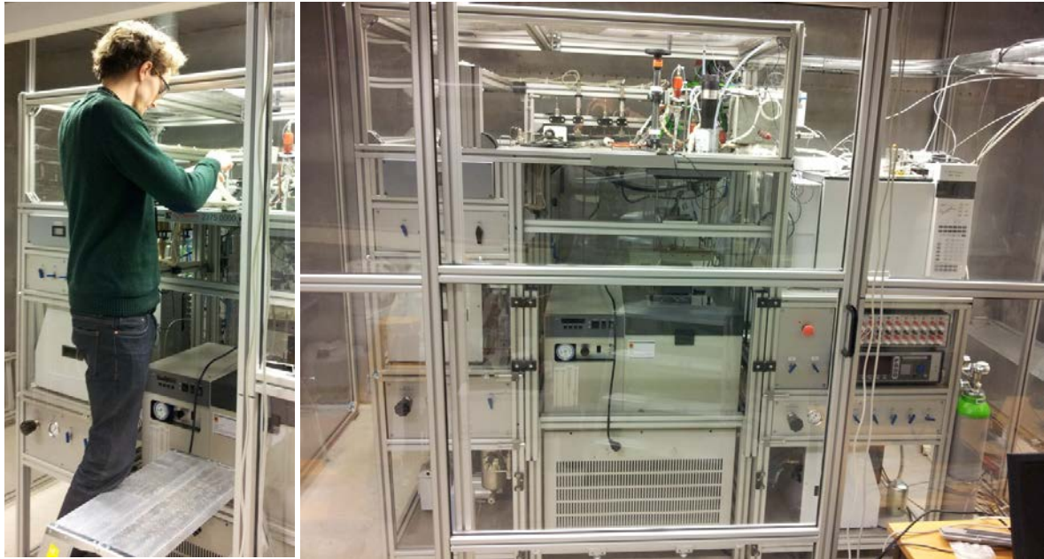
Fig. 1. Facilities of SINTEF ER for accurate phase equilibrium measurement using the analytical method developed in the CO 2 Mix project.
