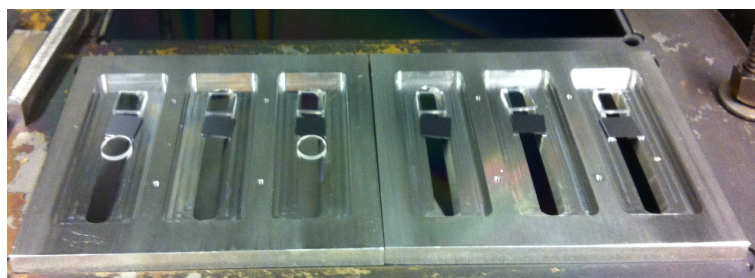
FIGURE 4.4: An image of the substrate holder used in the film depositions.
