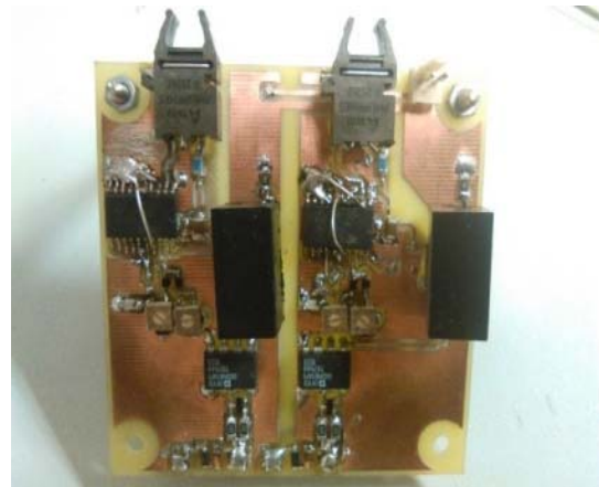
Fig. 3: Schematic diagram (a) and photo (b) of the gate driver with adjustable delays
