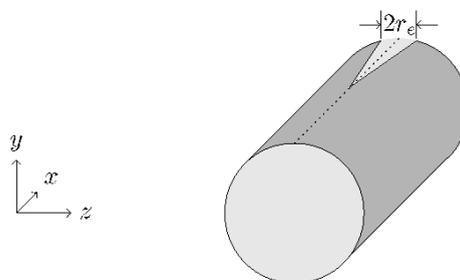
Figure 2. The crack propagates along the  $x$ -direction, leaving behind a growing opening of width  $2r_e(x)$  in the pipe. As the crack symmetrically propagates in both directions, only half of the domain is shown.
