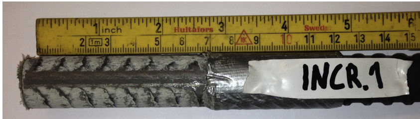
Fig. 9. 70 mm anchored length, pulled out after final testing. Shear failure in grout between ribs.
