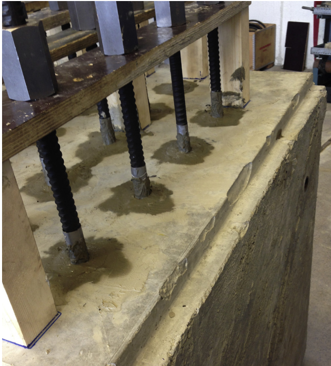
Fig. 5. Threaded steelbars installed in concrete block.
