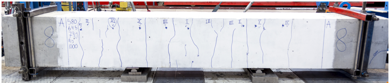
Figure E.16: Rissmønster for prisme 8- \phi 32-c40 for last 1012 kN
