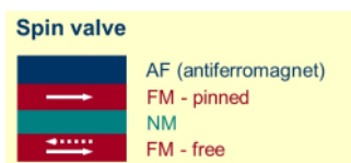
Figure 4.3: A model of a spin valve. The magnetization of the upper ferromagnetic layer is pinned by the antiferromagnet. The magnetization of the lower layer is free to move. The figure is from [23]
