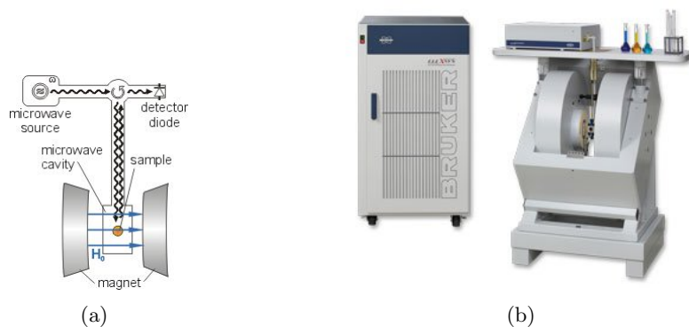
Figure 7.2: a) A schematic of the cavity based FMR setup. b) A photograph of the system used in the experiment, with the microwave source to the left and the magnet to the right.
