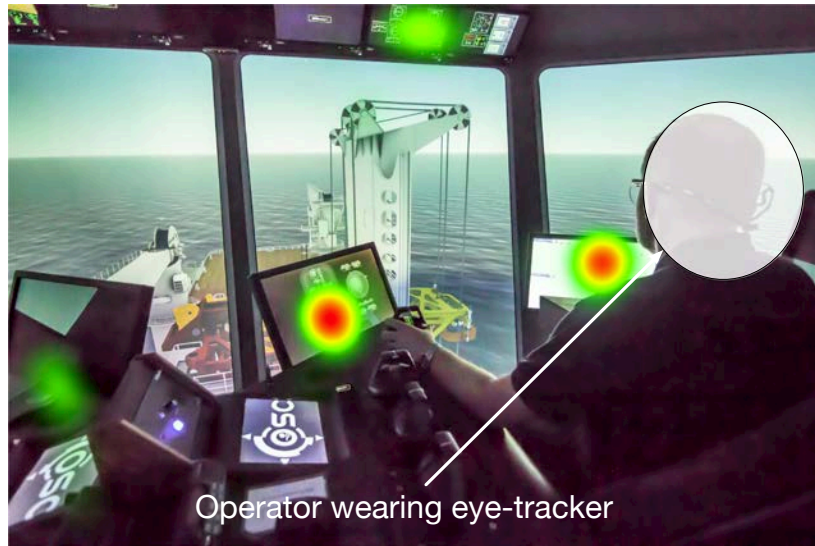
Figure 15: A heat map of the sub-routine performed in the bridge simulator station. Some elements of this figure are credit to the Offshore Simulator Centre AS (OSC), to Statoil and partners. Any person depicted in the image is being used for illustrative purposes only. People's faces are obscured for privacy concerns.
