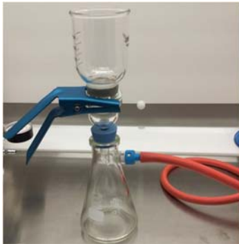
Figure 3: The filtration unit used for CWE. Photo by H. Vurucu.
