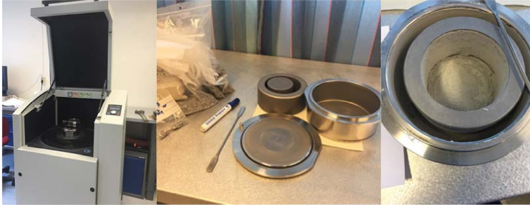
Figure 2: Vibratory disc mill RS 200 (Retsch). Photos by H. Vurucu.
