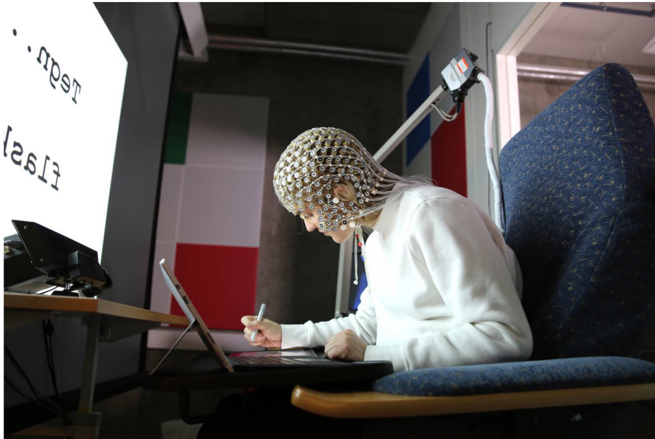
FIGURE 1 | Experimental set-up with a participant wearing the Geodesic Sensor Net. On the large screen right in front of the participant Pictionary™ words were projected that either had to be typed up, described in words, or drawn as pictures on one of the two laptop tablets in front of the participant using the keyboard (for typing and describing) or the stylus (for drawing).
