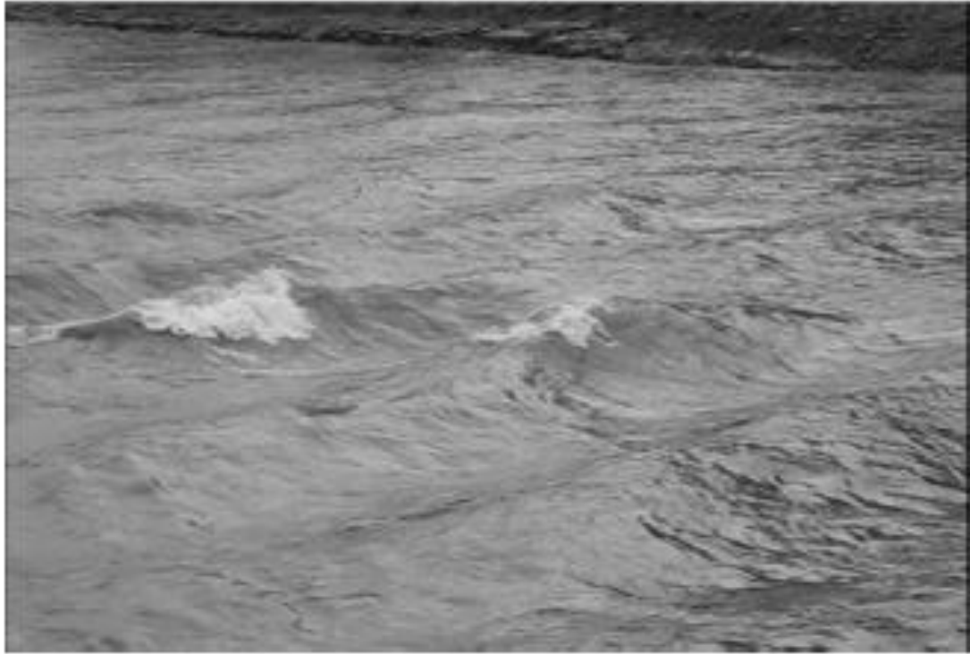
Figure 1. Partially breaking antidunes at the Bodendorf reservoir in Austria, during reservoir flushing (Olsen, 2013b).
