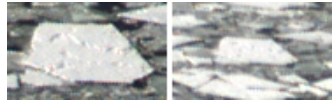
Fig. 10. Ice floe 5 in the reference camera image (left) and with a camera-to-object angle of 77.8^\circ (right).
