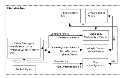
Fig. 7. The integration of the knuckle boom crane system modelling and simulations
