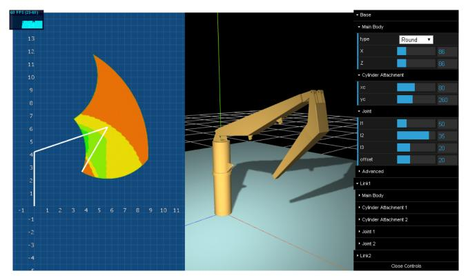
Fig. 3. A snapshot of the crane designer tool, workspace and load chart visualizations in a web browser
