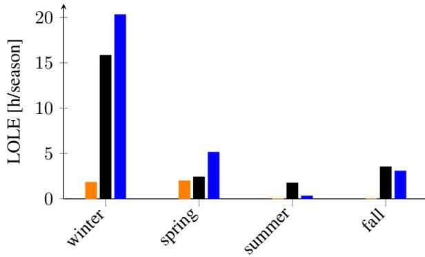
**Fig. 4.** The seasonal contribution to the LOLE's given in Table 2 for a typical wet, dry, and normal year. For instance, the sum of all the orange bars will give the LOLE for a dry year in Table 2.
