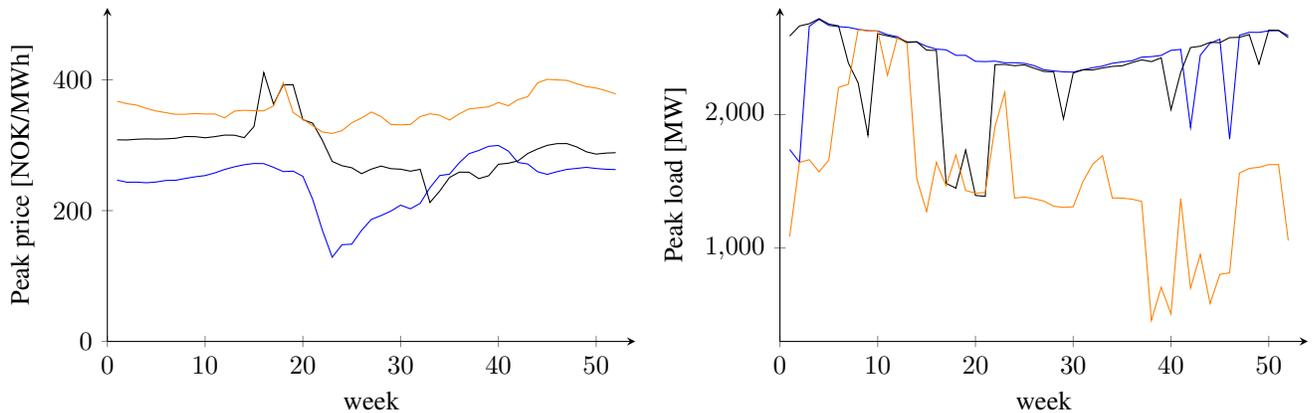
**Fig. 3.** Weekly values of peak price (left) and peak load (right) for a typical wet, dry, and normal year in southern Norway
