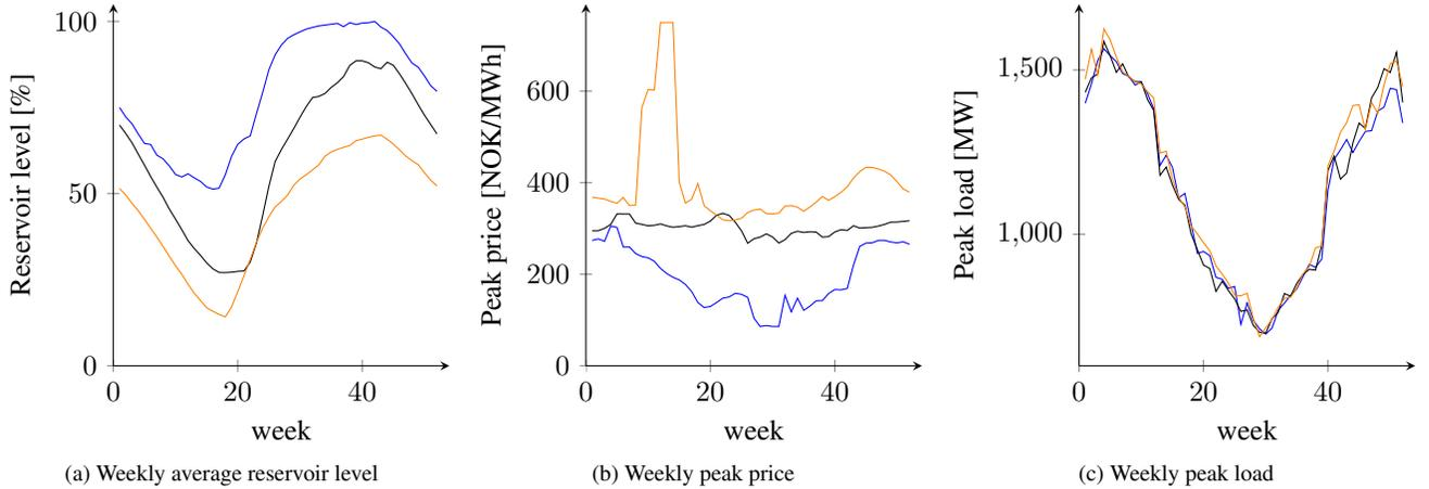
**Fig. 1.** Weekly values of average reservoir level, peak price, and peak load for a typical wet, dry, and normal year in Western Norway
