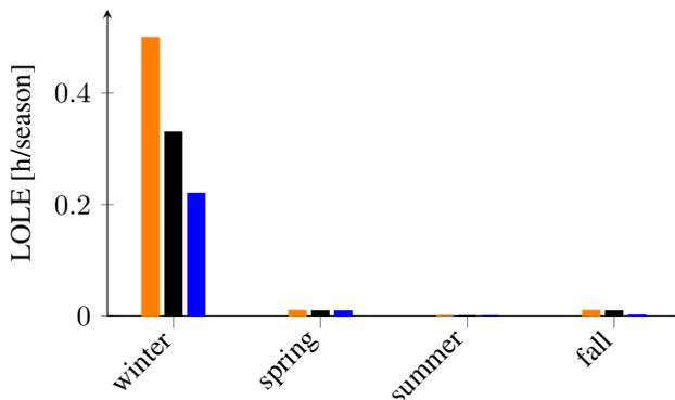
**Fig. 2.** The seasonal contribution to the LOLEs given in Table 1 for a typical wet, dry, and normal year. For instance, the sum of all the orange bars will give the LOLE for a dry year in Table 1.
