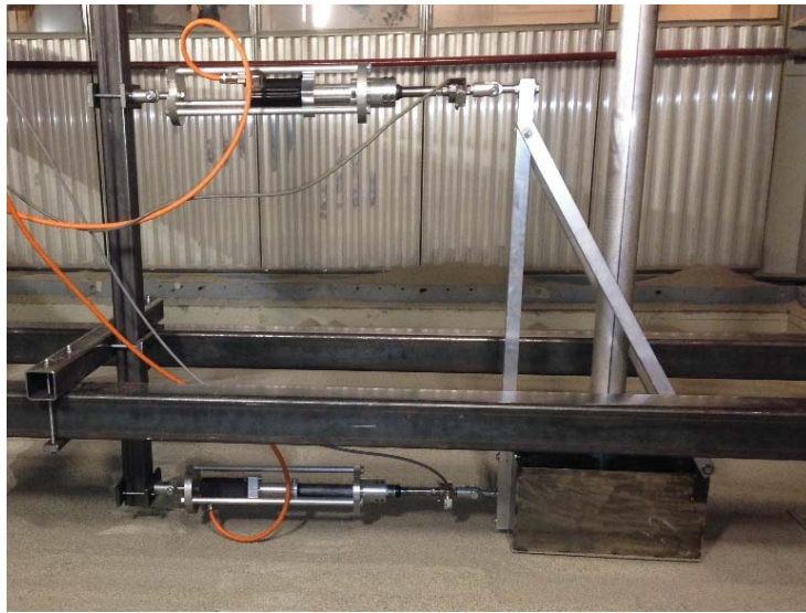
Figure 4-5. Left: Picture showing the prototype foundation in the sand bin. Right: schematic overview of prototype foundation, deformation application and load measurement arrangement.
