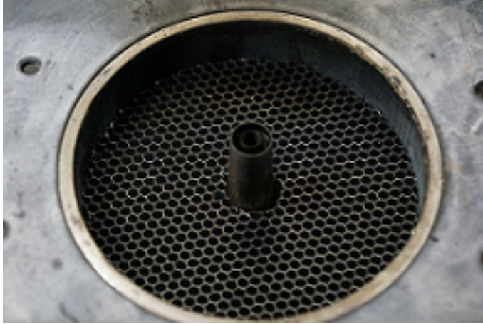
Figure 3.2: The nozzles where ethylene gas and air exits. The inner tube of exiting fuel gas has a 5 mm diameter and around this is an empty 10 mm diameter tube. Around these two nozzles is a 97 mm diameter circular tube of hexagonal array (honeycomb) where the airstream exits.
