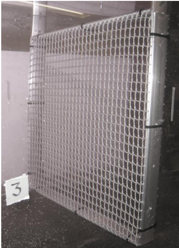
Figure 2. All nets were mounted in a frame made from oval aluminum profiles to minimize frame drag. Fitting curved aluminum profiles were used to clamp nets to the frame. Figure 1 shows the placement of the frame in the measurement setup.
