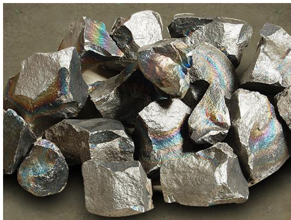
Figure 2.1: High-carbon ferromanganese. Photo reproduced from Marmara Metal (2016) .
