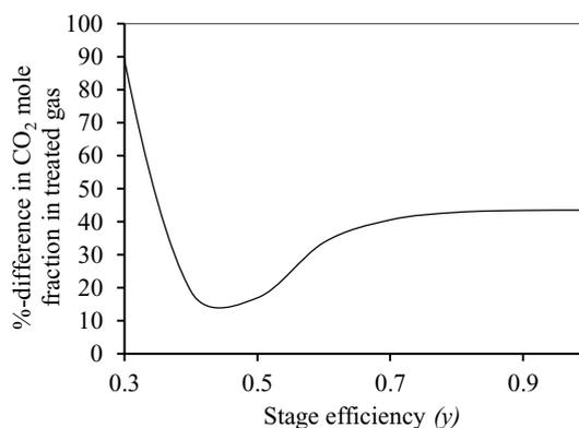
Fig. 4. Variation of difference of CO<sub>2</sub> mole fraction in the treated gas with changing stage efficiency (y) in the absorber.
