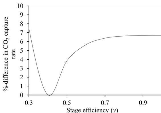
Fig. 3. Variation of difference of CO<sub>2</sub> capture rate with changing stage efficiency (y) in the absorber.
