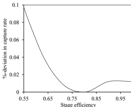
Fig. 5. Variation of difference of CO<sub>2</sub> capture rate with changing stage efficiency ( $\eta$ ) in the absorber.
