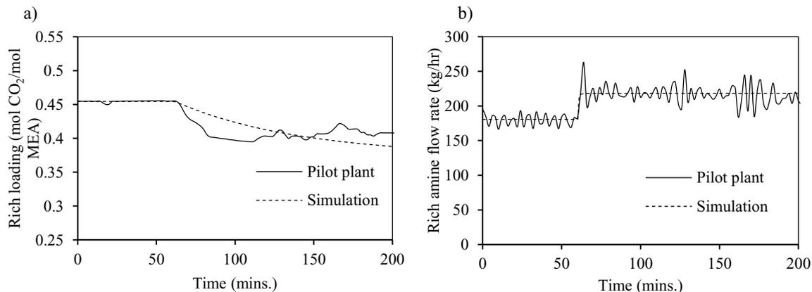
Fig. 9. a) Variation of rich loading and b) variation of rich amine flow rate: after applying step change in lean amine flow rate in the Gløshaugen pilot plant.
