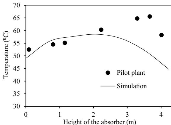
Fig. 6. Absorber temperature profile for case 2 with 0.4 as stage efficiency ( $\gamma$ ) in the absorber Gløshaugen pilot plant.
