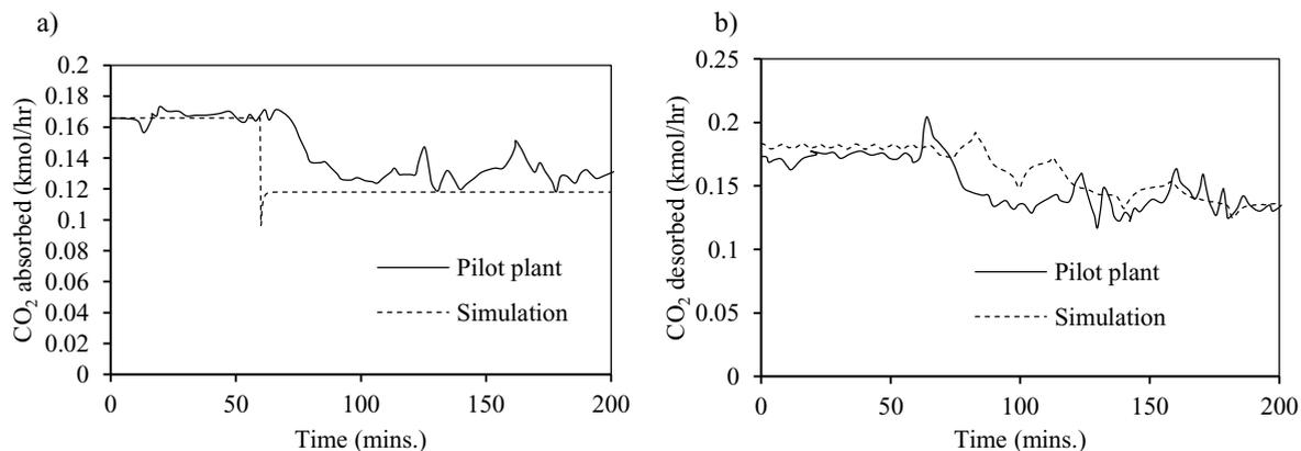
Fig. 10. a) Variation of absorbed and b) variation of desorbed  $\text{CO}_2$  flow rate: after applying step change in lean amine flow rate in the Gløshaugen pilot plant.
