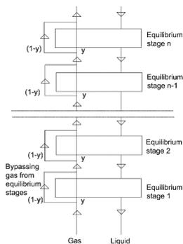
Fig. 1. Bypassing gas from equilibrium stages of absorber.
