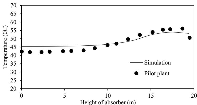
Fig. 8. Absorber temperature profile with 0.8 as stage efficiency in the absorber in Tiller pilot plant.
