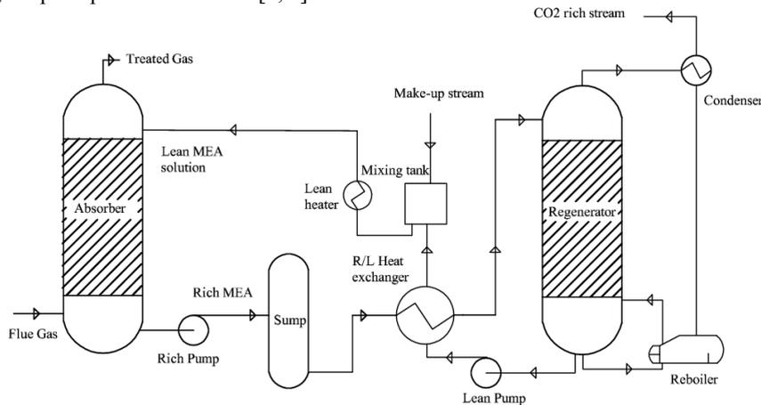
Fig. 2. Basic process flow-sheet of pilot plants.
