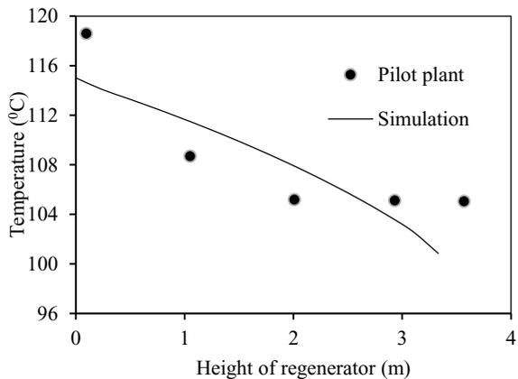
Fig. 7. Regenerator temperature profile for case 2 with 0.4 as stage efficiency ( $\gamma$ ) in the absorber in Gløshaugen pilot plant.
