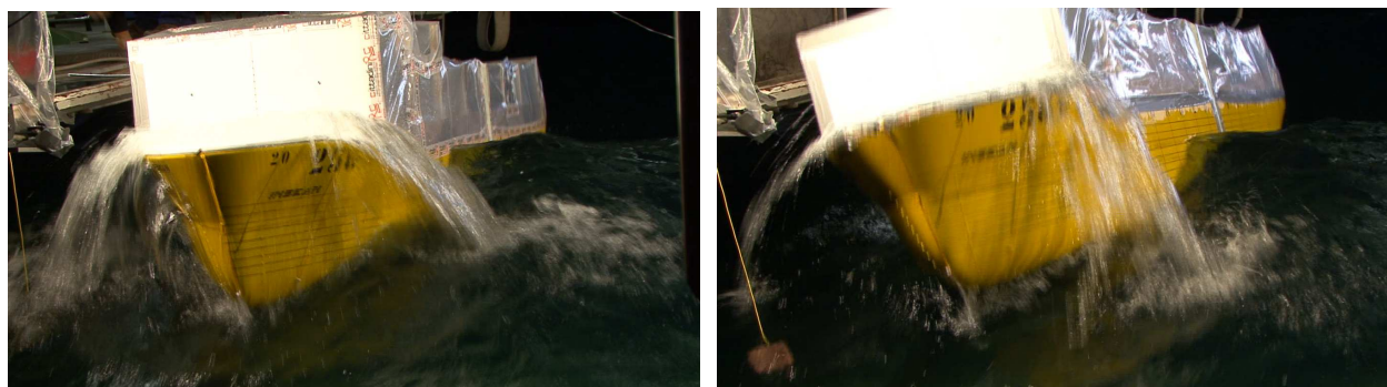
Figure 4: Nominal incident waves with \omega_{4n0}/\omega = 0.519 and kA = 0.25 : run 44 (left) and run 46 (right) at the time instant with wave crest at mid-ship.
