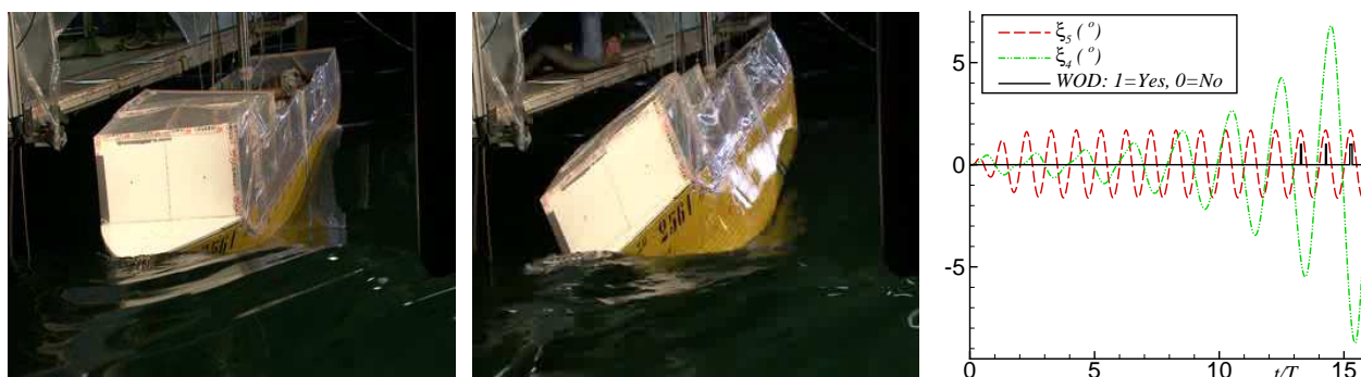
Figure 3: Nominal incident waves with \lambda/L = 0.75 and kA = 0.2 . Left and center: experimental snapshots before (left) and after (center) PR occurrence at the time instants with largest relative vertical motion at the bow. Right: numerical pitch, roll and WOD occurrence as a function of time.
