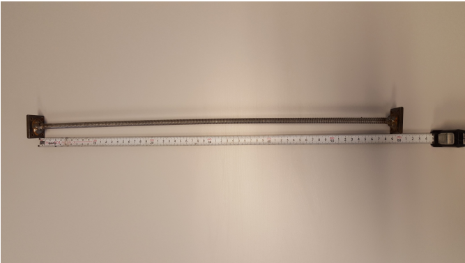
Fig. 2: Connecting rod with a measuring tape. By inspection the length of the rod is determined to be l_r = 596\text{mm} .
