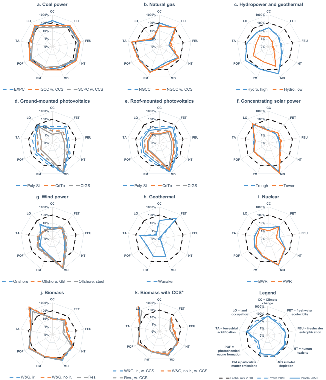
Fig. 1. Radar charts of environmental impacts of different types of power plants compared to the current global average power mix. *Biomass with CCS shows net negative greenhouse gas emissions, not shown on the logarithmic chart, the results range from -107\% to -122\% of the 2010 global electricity mix. EXPC: existing (subcritical) pulverized coal, IGCC: integrated combined cycle, SCPC: supercritical pulverized coal, NGCC: natural gas combined cycle, Poly-Si: polycrystalline silicon, CdTe: cadmium telluride thin-film, CIGS: copper indium gallium selenide, GB: gravity-based (concrete) foundation, BWR: boiling water reactor, PWR: pressurized water reactor, W & G: wood and grass, ir.: irrigation, Res.: forest residue.
