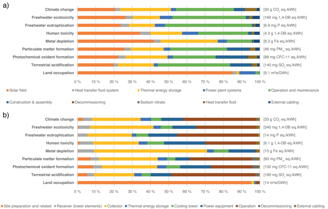
Figure S5: Contribution analysis of concentrated solar power: a) parabolic trough and b) central tower plants, under Africa & Middle East conditions (2400 kWh/m 2 a direct normal insolation).
