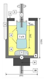
Figure 1. Schematic drawing of the experimental set-up. Dimensions in mm are in parenthesis. 1) rotating cathode connecting rod, 2) sintered alumina lid, 3) thermal couple, 4) Si<sub>3</sub>N<sub>4</sub> lining covering both ends, 5 a/b) carbon sample (cathode), a/b represents sample with/without slots, 6) electrolyte, 7) aluminum metal (100 g), 8) graphite crucible (anode), 9) graphite support, 10) anode lead.
