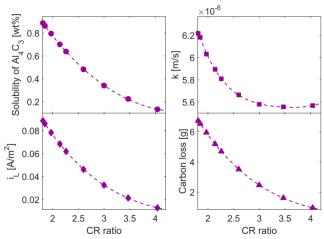
Figure 7. Solubility of Al<sub>4</sub>C<sub>3</sub>, mass transfer coefficient, k, limiting current density ( $i_L$ ), and carbon loss as a function of bath CR ratio. Caron loss is calculated based on 24 hours electrolysis in the present "inverted cell". Markers represent the calculated points and the dashed lines are polynomial fitting curves.
