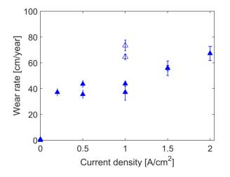
Figure 3. Wear rate as a function of current density for high graphitized carbon material at constant rotation speed of 50 rpm. Open triangle markers represent the tests without adding initial aluminum metal.
