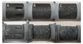
Figure 2. Appearance of tested cathode materials before (top) and after (bottom) 24 hours electrolysis at 1 A/cm current density and 125 rpm. A) high density graphitized, with slots B) graphitized and C) anthracitic.
