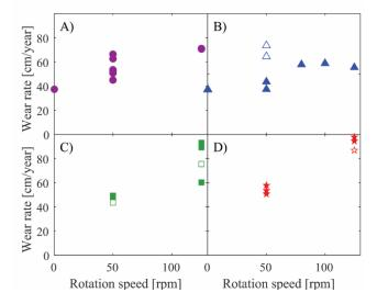
Figure 2. Average wear rates v.s. rotation speeds recalculated to cm/year for three types of cathode materials. A) high density graphitized, B) high density graphitized with slots, open triangle markers represent tests without initial aluminum present in the cell, C) graphitized. Open square and star markers represent the cylinder samples with slots.
