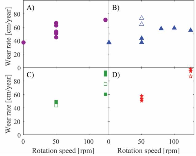
Figure 2. Average wear rates v.s. rotation speeds recalculated to cm/year for three types of cathode materials. A) high density graphitized, B) high density graphitized with slots, open triangle markers represent tests without initial aluminum present in the cell, C) graphitized. Open square and star markers represent the cylinder samples with slots.
