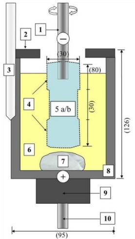
Figure 1. Schematic drawing of the experimental set-up. Dimensions in mm are in parenthesis. 1) rotating cathode connecting rod, 2) sintered alumina lid, 3) thermal couple, 4) Si<sub>3</sub>N<sub>4</sub> lining covering both ends, 5 a/b) carbon sample (cathode), a/b represents sample with/without slots, 6) electrolyte, 7) aluminum metal (100 g), 8) graphite crucible (anode), 9) graphite support, 10) anode lead.
