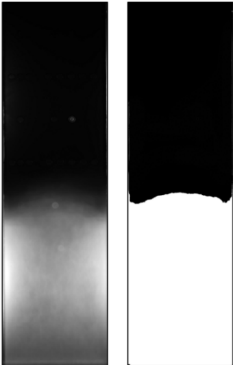
Figure 3: An example of the experimental volume fraction plot averaged from 200 images (left) as well as the approximated 10% volume fraction threshold (right).
