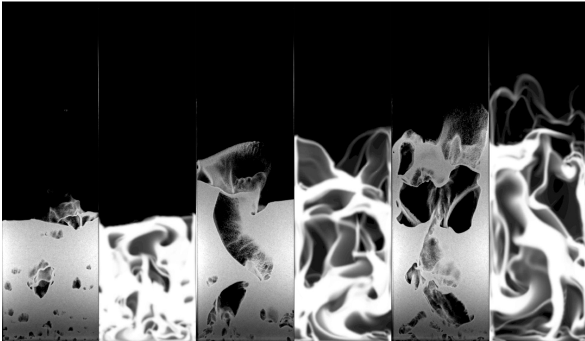
Figure 7: Visual comparison of the bed dynamics of the experiments and the simulations as the fluidization velocity is increased. The three pairs of images from left to right are from cases 9, 15 and 10.
