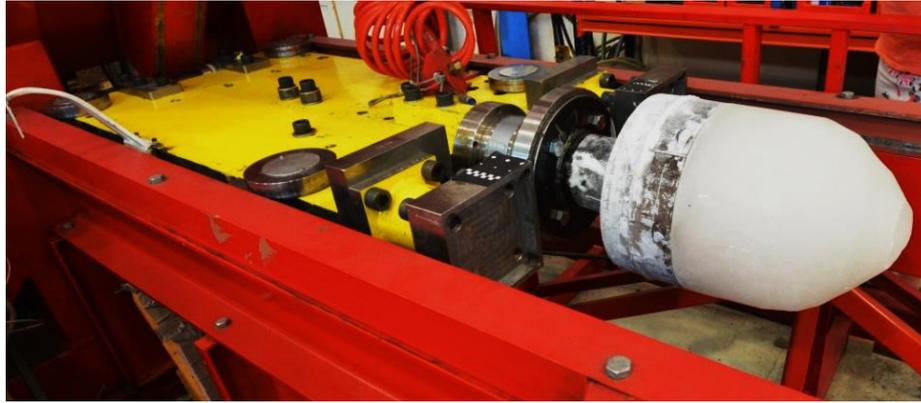
Figure 1 Ice sample mounted to the trolley.
