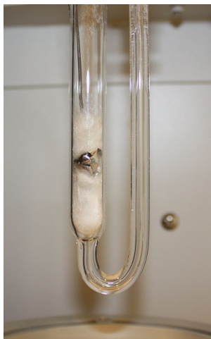
Figure 4.6: Palladium alloy membrane in a glass reactor between quartz wool. On the end of the thin black metal bar seen behind the glass reactor, the thermocouple is localized which is in proximity of the membrane.
