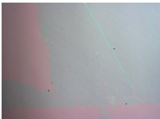
(c) After 2 hours in acetone to remove PMMA
