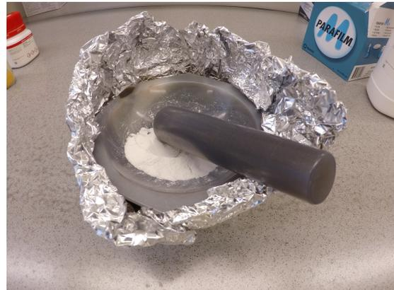
(b) Mortar used to finely grind and mix powder
