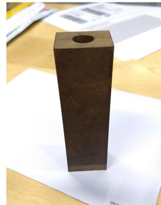
(e) Mould for annealing the glass
